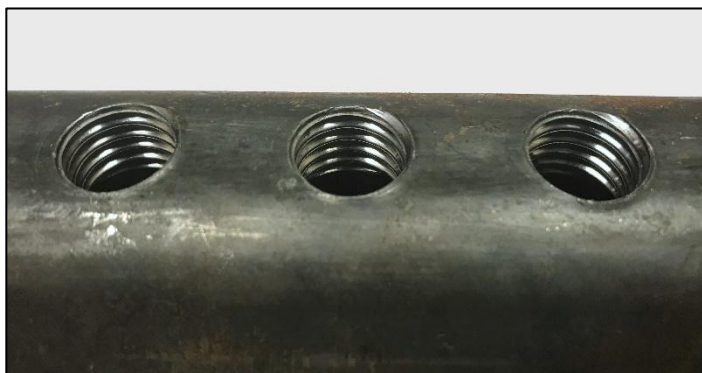
FIGURE 5: Clean Acceptable Coupler
