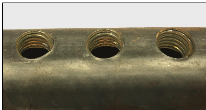
FIGURE 6: Unacceptable Rust in Coupler Threads
