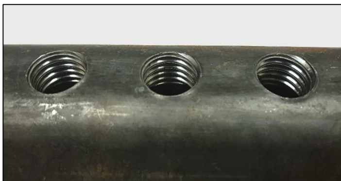
FIGURE 5: Clean Acceptable Coupler
