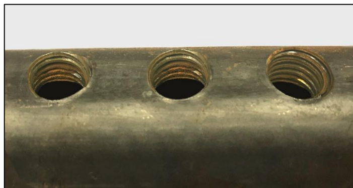
FIGURE 6: Unacceptable Rust in Coupler Threads
