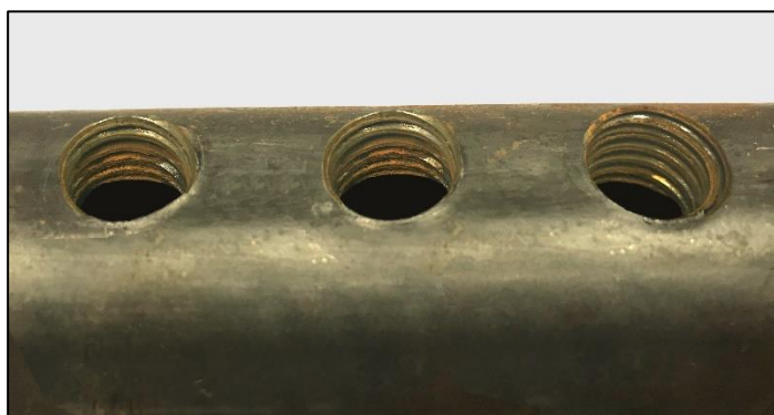
FIGURE 6: Unacceptable Rust in Coupler Threads
