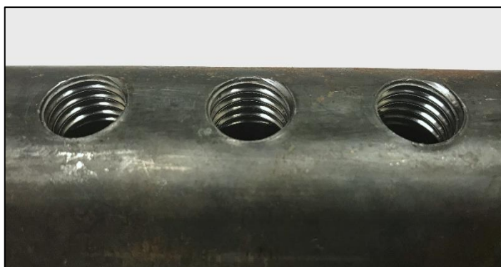
FIGURE 5: Clean Acceptable Coupler
