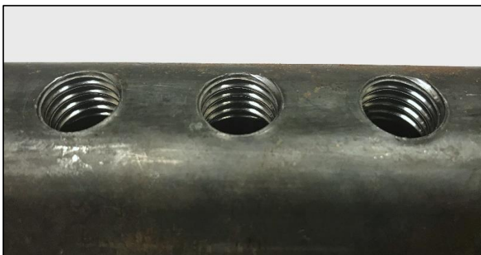
FIGURE 5: Clean Acceptable Coupler
