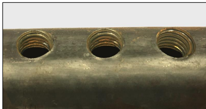
FIGURE 6: Unacceptable Rust in Coupler Threads
