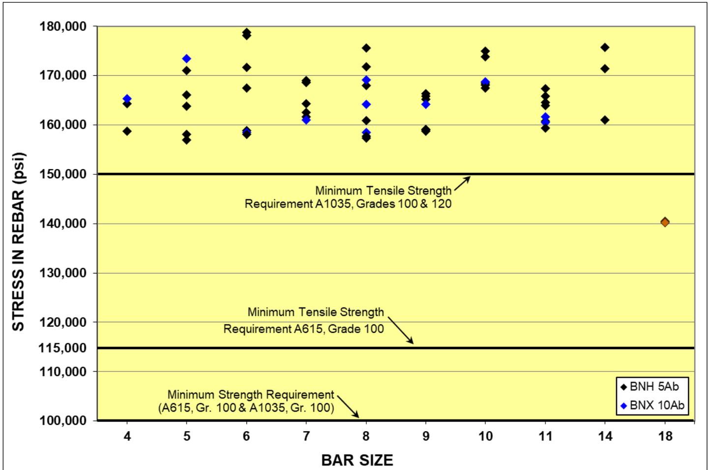
◆ 18BNH tests stopped at 140ksi proof load due to machine limitations.
